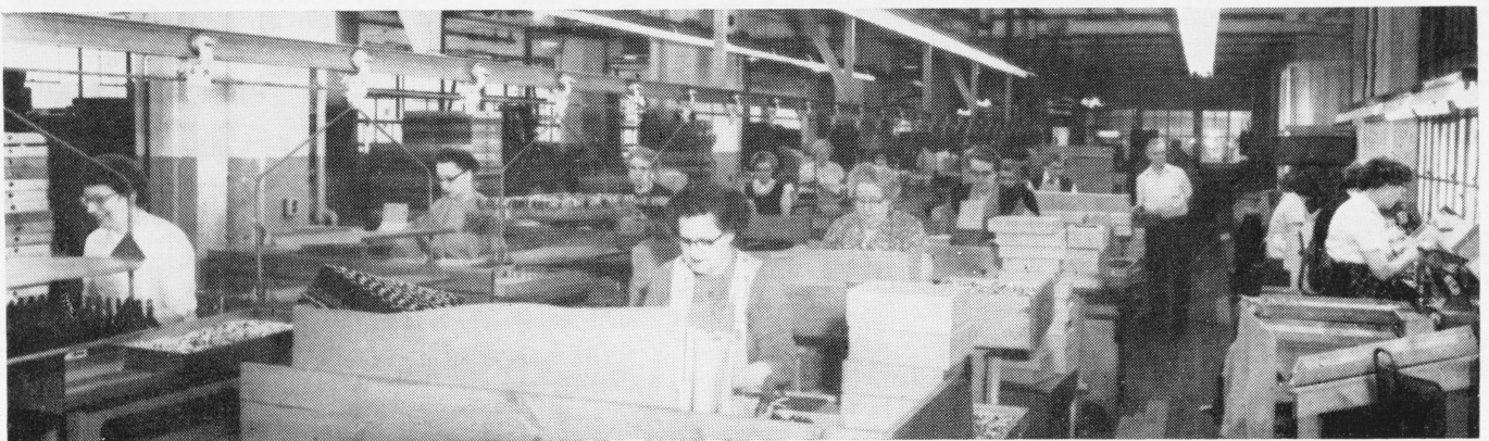
END OF THE LINE. The central conveyor moves on the overhead rail running between the assembly benches. Here,
